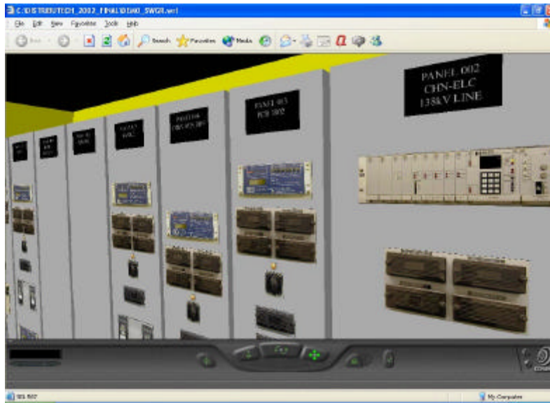
Figure 7. VRML Switchgear Control Room Detail
